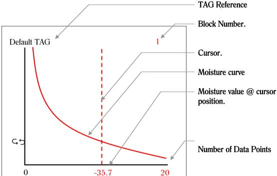
Pressing the 'A' and 'V' keys moves the cursor along the X-axis of the graph. The Moisture value printed in the middle of the X-axis changes to indicate the value at the point where the cursor crosses the moisture curve.
