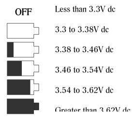
The Icon fills from the left when the external power supply is connected. This indicates that the battery is receiving a charging current and should be fully charged within 14 hours.
