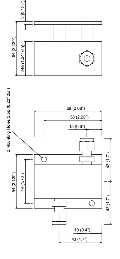
NOTE. The Assembly is shown with 1/4" OD tube fittings. The dimension across the tube fittings will vary for all other size fittings.
