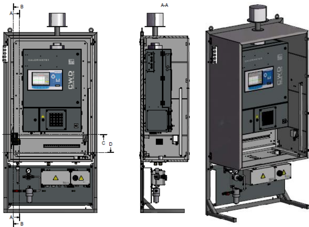
Fig. 1.2: System overview, protective housing with combustion calorimeter
