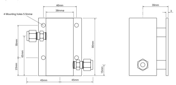
Note: The Assembly is shown with 1/4@ OD tube fittings. The dimensions across the tube fittings will vary for all other size fittings.
