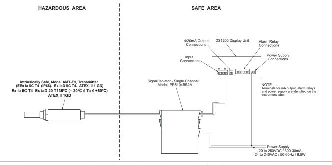
Model AMT-Ex Dewpoint Transmitter Using PR5104BB2B Dual Isolator and Model DS1200 Display
